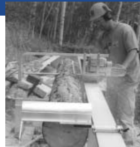
Left to right: Phil Gould takes a slab cut off a log with his Logosol. He shows off a board in the center photo. Above right: With no throttle lock on his chainsaw, Phil Gould uses two hands to run his mill.
