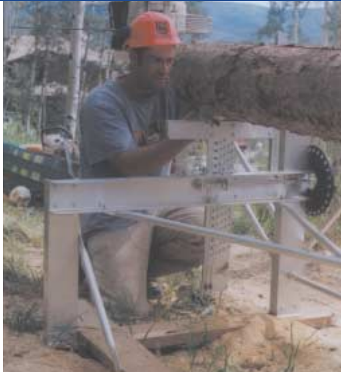
Phil Gould measures the center of a log. By adjusting the two scale plates, he can saw tapered logs.
