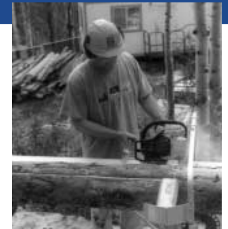
Left to right: Phil Gould takes a slab cut off a log with his Logosol. He shows off a board in the center photo. Above right: With no throttle lock on his chainsaw, Phil Gould uses two hands to run his mill.
